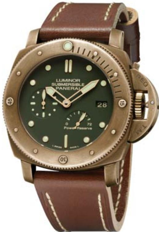
**Movement:** Automatic mechanical, Panerai P.9002 calibre, executed entirely by Panerai, 13 $\frac{3}{4}$  lignes, 7.9 mm thick, 29 jewels, Glucydur® balance, 28,800 alternations/hour. Incabloc® anti-shock device. Power reserve 3 days, two barrels. 237 components.
