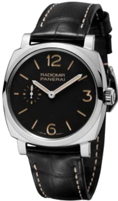
**Movement:** Hand-wound mechanical, Panerai P.999/1 calibre, executed entirely by Panerai, 12 lignes, 3 mm thick, 19 jewels, Glucydur® balance, 21,600 alternations/hour. Incabloc® anti-shock device. Power reserve 60 hours. 144 components.
