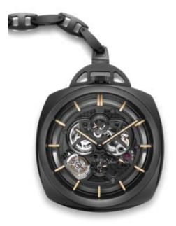
Movement: Skeleton hand-wound mechanical, Panerai P.2005/S calibre, executed entirely by Panerai, 161/4 lignes, 10.05 mm thick, 31 jewels, Glucydur® balance, 28,800 alternations/hour. KIF Parechoc® anti-shock device. Power reserve 6 days, three barrels. 277 components.
